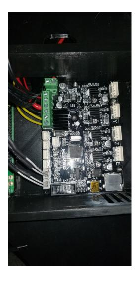
9) Next, with your extended limit switches from set 5, you will route them though the new case, and into your mainboard where the labels are. (see image under step 6 for any clarification) Once everything is lined up it should look like the image below.
