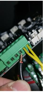
8) Once you have completed the bare wire extensions (no JST connectors) you have to extend the Bed and Hot End thermistors. You want to mark one side of the wire, cut that side, splice one of the black wires that you cut earlier from step 2, then once its shrink wrapped you can move on to the other half of the connector. I am not sure if polarity matters but to play it on the safe side I made sure to keep the original polarity. It should look like this once you are finished with this step.
