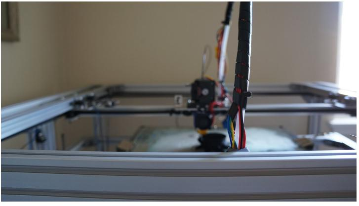
The umbilical cord will likely lay down, but that doesn't seem to be an issue. It is important that you make sure there is enough tubing so you don't constrain the extruder carriage.
