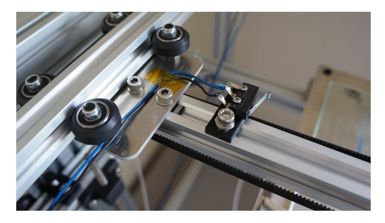
Y end stop is located on the left side of the extruder beam.
