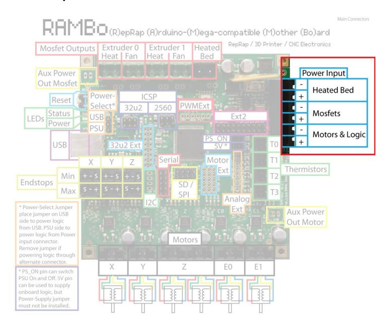
**CAUTION:** Be sure to wire to the correct polarity (positive/negative) or you will damage the board.
