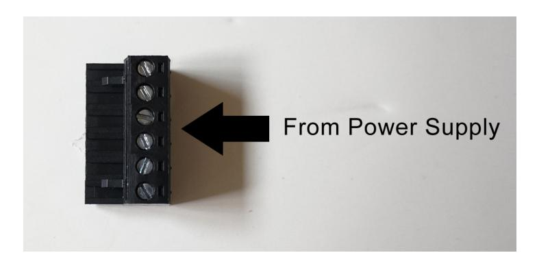
The screw terminal connector above is part of your controller kit (in a bag). Note that it is keyed and will only insert one way.
