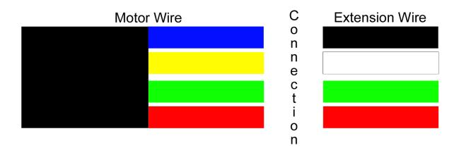
Since the wire colors of the motor and the shielded cable do not match, use the conversion above.
