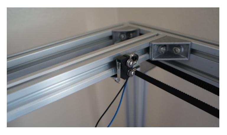
The X endstop is located at the back right corner of the printer.
