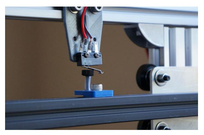
The Z end stop components include the end stop switch assembly and the adjustable end stop.
