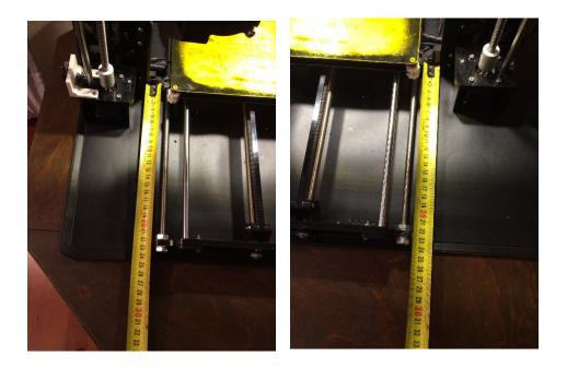
2. Measure left and right back to midsection, if the numbers are different loosen the nuts and make them exactly the same.
