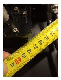
4. Crossmeasure from left back frame corner to right front motor mount, compare the number with measurement in point 3.
