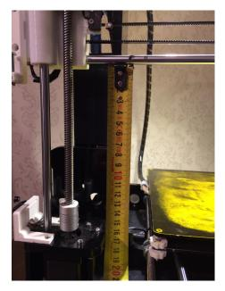
8. Measure from right motormount to the guide bar, compare the numbers with measurement in point 7. If they differs just turn the threadbar until the distance is the same on both sides.
