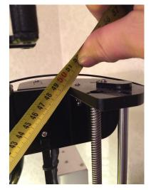
Crossmeasure from right motor mount to left top frame corner, compare the number with measurement in point 5.
