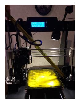
To make shure that x-axis guide bars are leveled to the frame (do not use water level) Measure from left motor mount to the guide bar, note the measurement.
