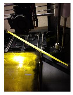
Crossmeasure also from left bottom to right top Measure from motormount corner to top frame corner and note the number.
