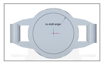
The original Lego-part has the following draft-angles: inside = 0.8deg / outside = 0.2deg
