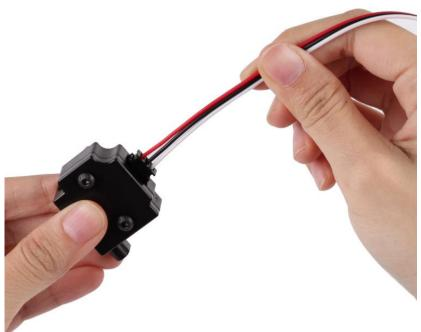
Connect sensor with the 4-pins port to the 3d printer via the white port shown in the below image.
